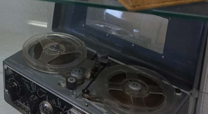
NAGRA NAGRA I (CERA 200) The NAGRA I is one of the original 1/4 inch cassettes made at the beginning of the NAGRA history. Mechanically driven with battery powered tape transport.
