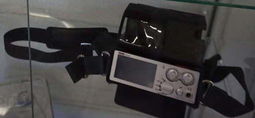
NAGRA NAGRA VI (2008 - ) 8-channel digital recorder using both internal hard disk and removable compact flash media. Includes a built-in mixer and full TC system. Designed for both music and film / TV applications. Available in 4 different colors.
