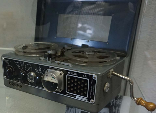
NAGRA NAGRA II (1953-1955) Introduced in 1953, 7,000 NAGRA II machines were manufactured. In 1953 the "II" version with printed circuit boards was designed. Also mechanically driven with battery powered tube electronics.
