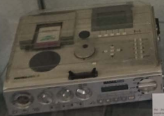
NAGRA NAGRA D / DK (1992 - 2004) A 24 bit, 48kHz digital recorder using three head technology. Used primarily for CD mastering and feature film production. This was the first portable multi-track digital recorder.
